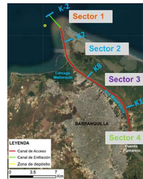
Figure 2-3 Access channel map and description of sectors. Source: Own elaboration with information from Cormagdalena.
