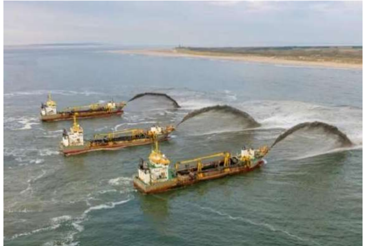
Figure 3-3: Typical methods for spreading marine sediments on sea and coastal areas. Source: Dutch Department of Waterways and Public Works
