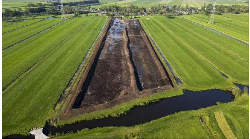
Figure 2-7: Typical Dutch sediment drying depot from above. Source: bodembreed.
